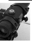
The standard targeting scope uses three reticle red dots to represent distances of 20, 40, and 60 yards. Two calibrated screws on the scope allow you to adjust sighting. The top screw adjusts horizontally (windage); the side screw adjusts vertically (elevation).
