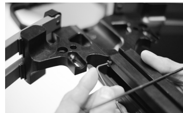
Figure 5: Attaching stock assembly to top side of riser
